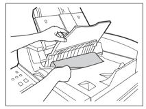
Lifting the handle in the direction of the arrow, pull it toward you.
